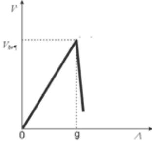
**Figure 1.** Cross-sectional force-displacement diagram for brittle elements
