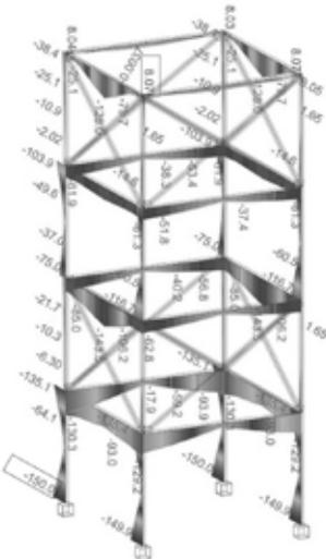
**Figure 13.** Envelop diagram (min. value) of earthquake moments after plastic redistribution, kNm.
