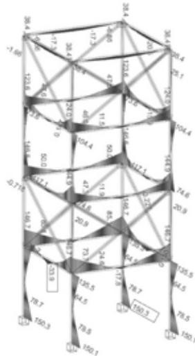
**Figure 14.** Envelop diagram (max. value) of earthquake moments after plastic redistribution, kNm.
