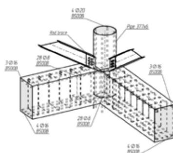
**Figure 8.** View of the frame assembly
