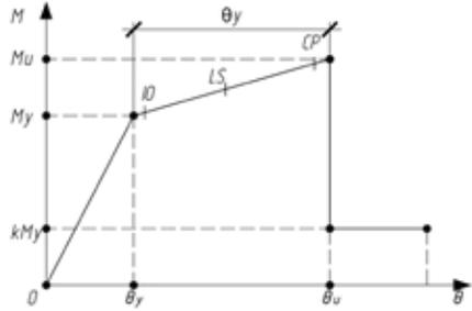
**Figure 2.** Moment-angle diagram for a plastic element
