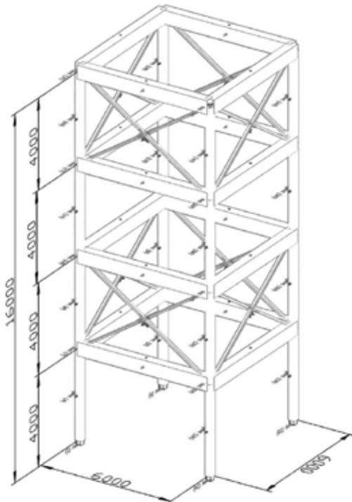
Figure 3. Composite three-dimensional frame
