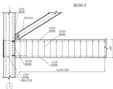
**Figure 7.** Drawings of the frame assembly structures
