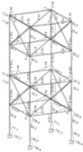
**Figure 11.** Envelop diagram (max. value) of earthquake moments, kNm.
