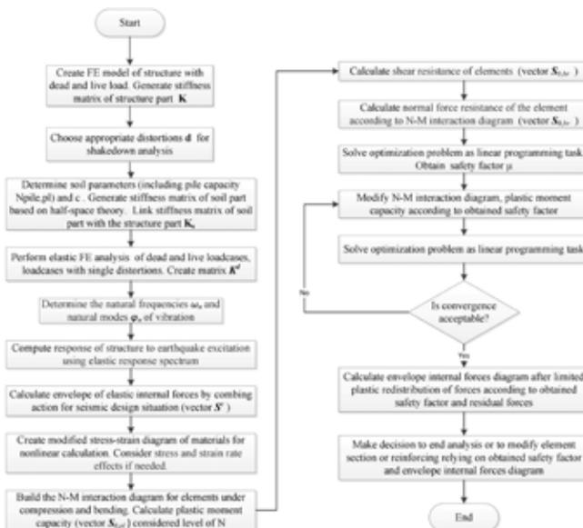
**Fig. 15.** General block diagram of shakedown analysis for earthquake effects
