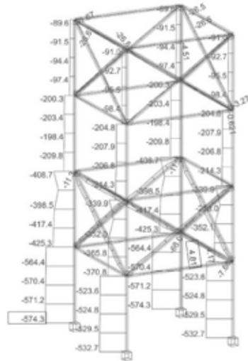
**Figure 10.** Envelop diagram (min. value) of longitudinal forces, kN.
