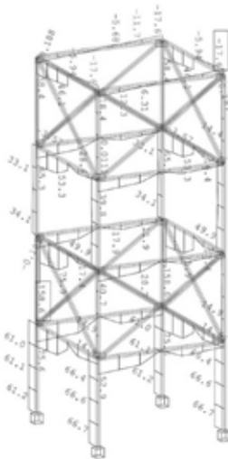
**Figure 9.** Envelop diagram (max. value) of shear forces, kN.
