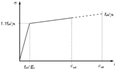
**Figure 5.** Deformation diagram for reinforcing steel
