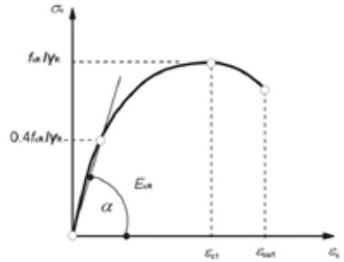
**Figure 6.** Deformation diagram for concrete
